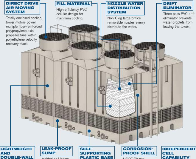
Plastic is lighter than conventional cooling towers and integrated double-wall is more than 10 times the average wall thickness of metal towers.
