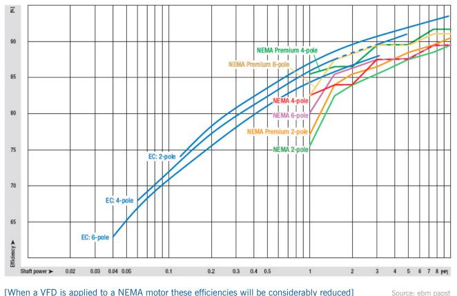
[When a VFD is applied to a NEMA motor these efficiencies will be considerably reduced]
