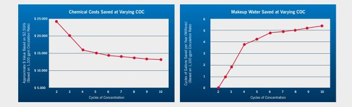
Utilizing components with greater corrosion resistance can permit operation at higher cycles of concentration which can significantly reduce water usage, water blowdown, and chemical usage.
